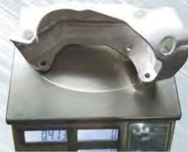
New two pieces welding motor bracket
