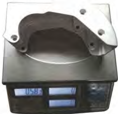
Traditional one piece forging motor bracket Weight: 583g
