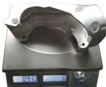
New two pieces welding motor bracket Weight: 413g
