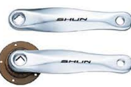
SS-7002 Crank: Forged 6061/T6 alloy Length: 170mm Size: 1/8"x5 holes Diam: Ø1.37
