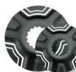
SPIDER: D2 (Ø110 / Ø95) MATERIAL: FORGED AL-6061-T6 FINISH: BLACK SAND ANO. WEIGHT: 49G (Ø110) 33.5G (Ø95)
