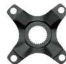
SPIDER: S1 (29T) MOUNTING INTERFACE: 29T MATERIAL: AL-6061-T6 FINISH: BLACK SAND ANO. BCD: 104MM
