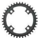
NW-38T CHAINRING MATERIAL: AL-7075-T6 CHAINRING FINISH: BLACK SAND ANO. BCD: 104MM
